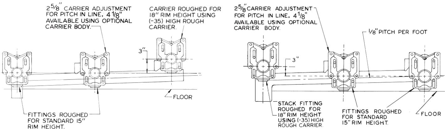
The above shows an installation utilizing a JOSAM vertical fitting and carrier and a horizontal waste line with fittings and carriers. The horizontal fitting and carrier on the end show the (-35) high rough for wheelchair use.
