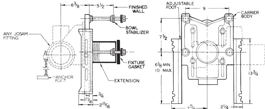
(-35) Option Carrier can be used with all adjustable fittings. When used with blowout closets over 12 1/2", specify -M1358.
