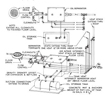
Oil separator recessed flush with floor, servicing a floor drain. Flow control is installed with cleanouts to facilitate servicing.
