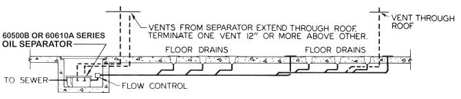
Oil separator and flow control installed in pit, servicing a battery of floor drains.
