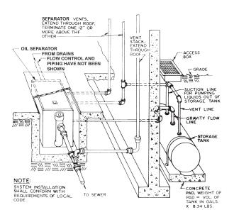
Typical arrangement of separator, draw-off piping, venting and oil storage facility.
