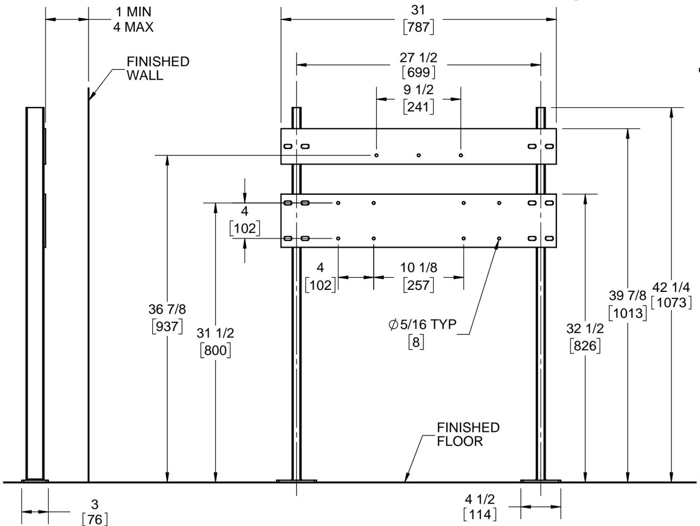
JOSAM RECOMMENDS - FEET BE SECURED TO FLOOR WITH 1/2" BOLTS AND ANCHORS BY OTHERS
