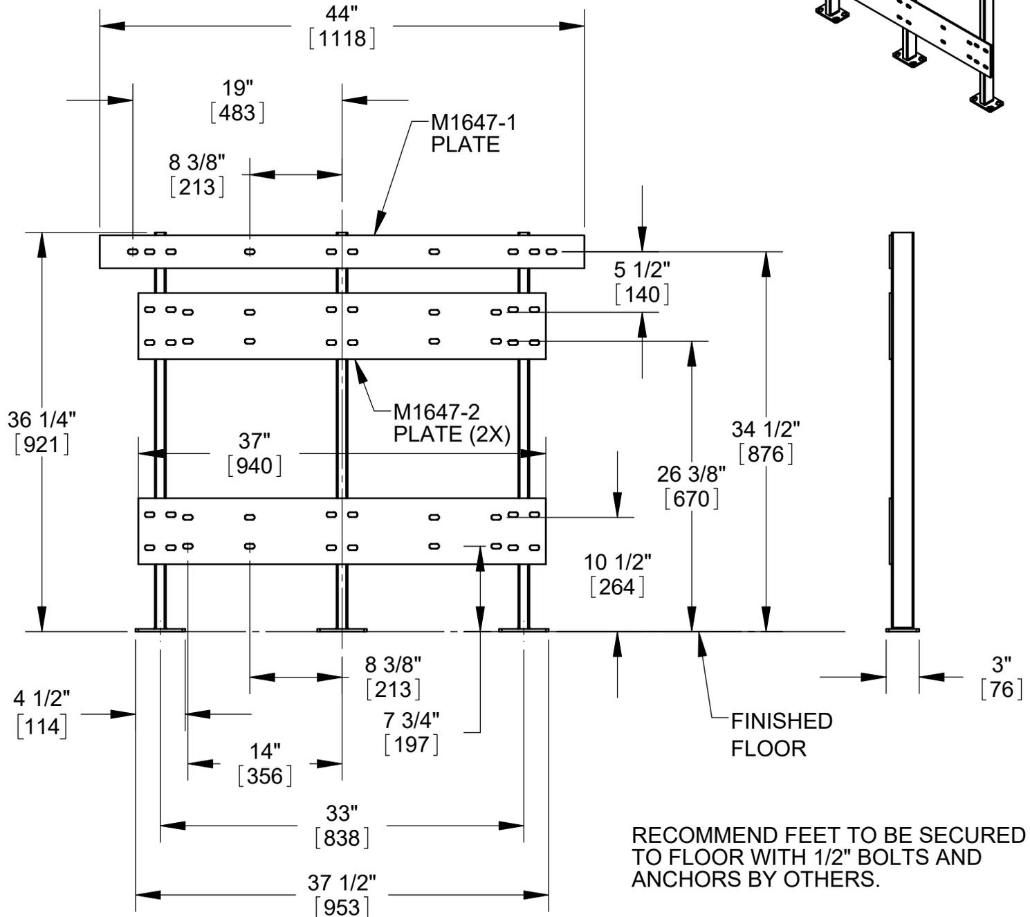
RECOMMEND FEET TO BE SECURED TO FLOOR WITH 1/2" BOLTS AND ANCHORS BY OTHERS.
