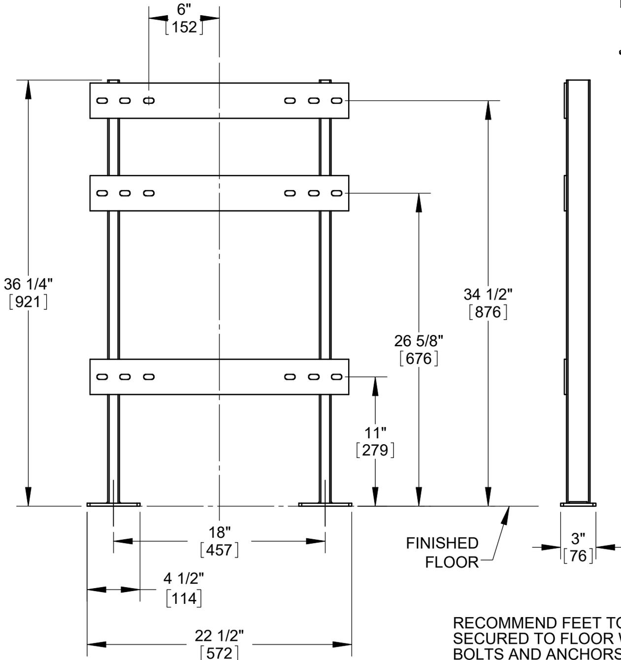
RECOMMEND FEET TO BE SECURED TO FLOOR WITH 1/2" BOLTS AND ANCHORS BY OTHERS
