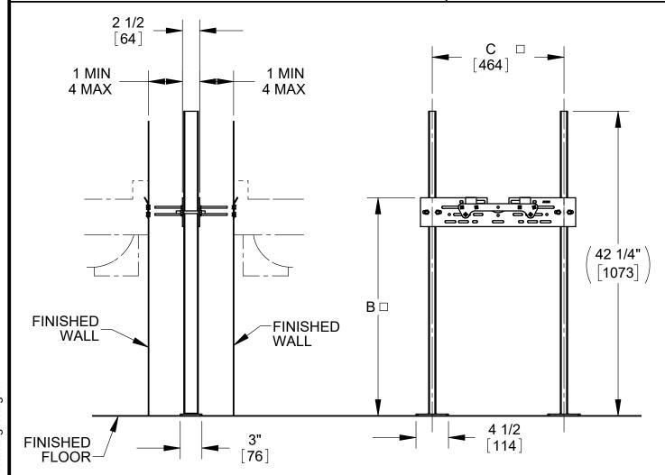
JOSAM RECOMMENDS - FEET BE SECURED TO FLOOR WITH 1/2" BOLTS AND ANCHORS BY OTHERS.
