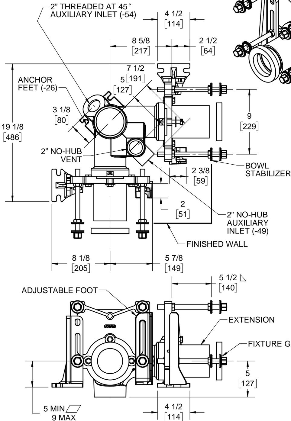
△ FOR DIMENSION SHORTER THAN 5-1/2" (1-3/4" MIN) CUT EXTENSION. FOR LONGER EXTENSION (10-1/2" MAX) SPECIFY (-10).
