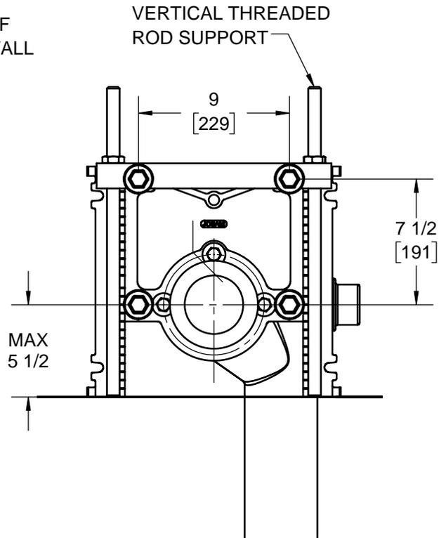
RECOMMEND CONCRETE ANCHORS WITH 750 LBS. PULL-OUT FORCE EACH
