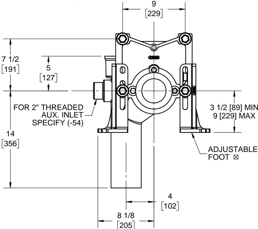
▽ FOR DIMENSION SHORTER THAN 5-1/2" (1" MIN) CUT EXTENSION FOR LONGER EXTENSION (10-1/2" MAX) SPECIFY (-10).
