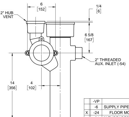
$\geq$  FOR DIMENSION SHORTER THAN 5-1/2" (1" MIN) CUT EXTENSION. FOR LONGER EXTENSION (10-1/2" MAX) SPECIFY (-10)
