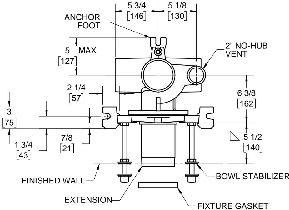
△ FOR DIMENSION SHORTER THAN 5-1/2" (1" MIN) CUT EXTENSION. FOR LONGER EXTENSION (10-1/2" MAX) SPECIFY (-10)
