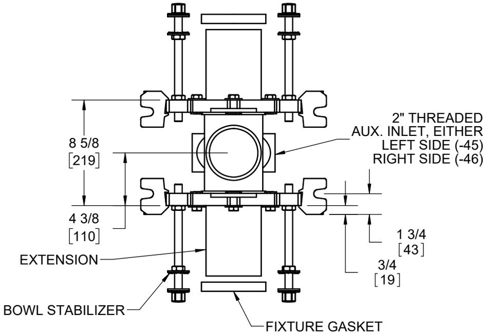
△ FOR DIMENSION SHORTER THAN 5-1/2" (1" MIN) CUT EXTENSION FOR LONGER EXTENSION (10-1/2" MAX) SPECIFY (-10).
