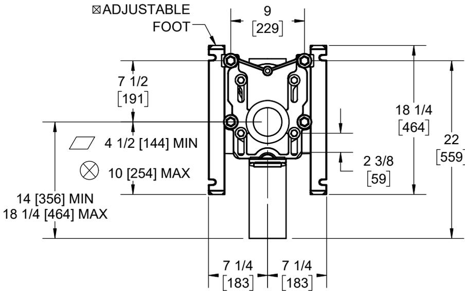
△ FOR DIMENSION SHORTER THAN 5-1/2" (1" MIN) CUT EXTENSION. FOR LONGER EXTENSION (10-1 1/2" MAX) SPECIFY (-10)
