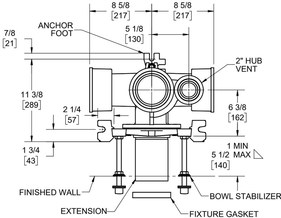
▽ FOR DIMENSION SHORTER THAN 5-1/2" (1" MIN) CUT EXTENSION. FOR LONGER EXTENSION (10-1/2" MAX) SPECIFY (-10)
