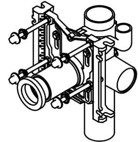
▽ FOR DIMENSION SHORTER THAN 5-1/2" (1" MIN) CUT EXTENSION. FOR LONGER EXTENSION (10-1/2" MAX) SPECIFY (-10)
