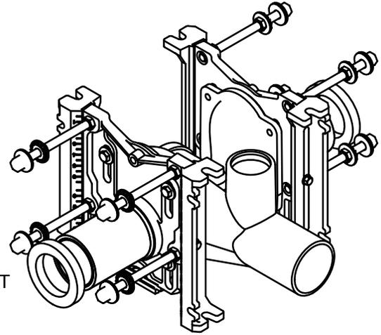
△ FOR DIMENSION SHORTER THAN 5-1/2" (1" MIN) CUT EXTENSION. FOR LONGER EXTENSION (10-1/2" MAX) SPECIFY (-10)
