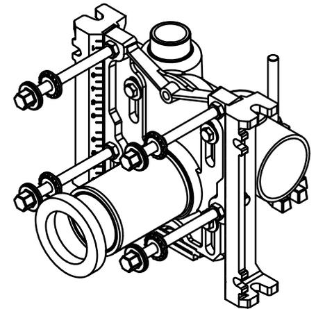
▽ FOR DIMENSION SHORTER THAN 5-1/2" (1" MIN) CUT EXTENSION. FOR LONGER EXTENSION (10-1/2" MAX) SPECIFY (-10)
