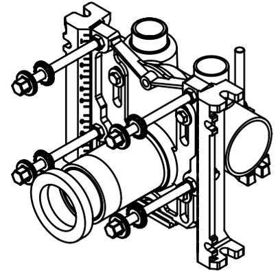
△ FOR DIMENSION SHORTER THAN 5-1/2" (1" MIN) CUT EXTENSION. FOR LONGER EXTENSION (10-1/2" MAX) SPECIFY (-10)
