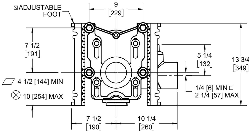
△ FOR DIMENSION SHORTER THAN 5-1/2" (1" MIN) CUT EXTENSION. FOR LONGER EXTENSION (10-1/2" MAX) SPECIFY (-10).
