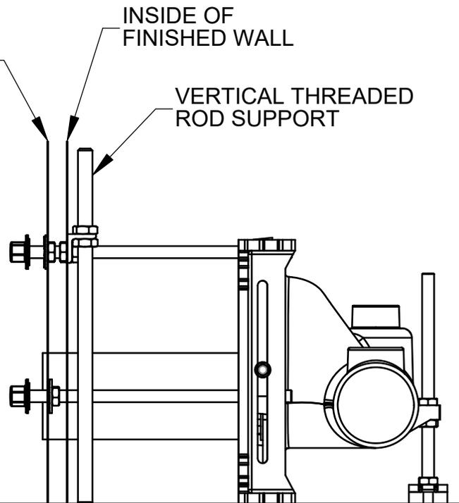
RECOMMEND CONCRETE ANCHORS WITH 750 LBS. PULL-OUT FORCE EACH.
