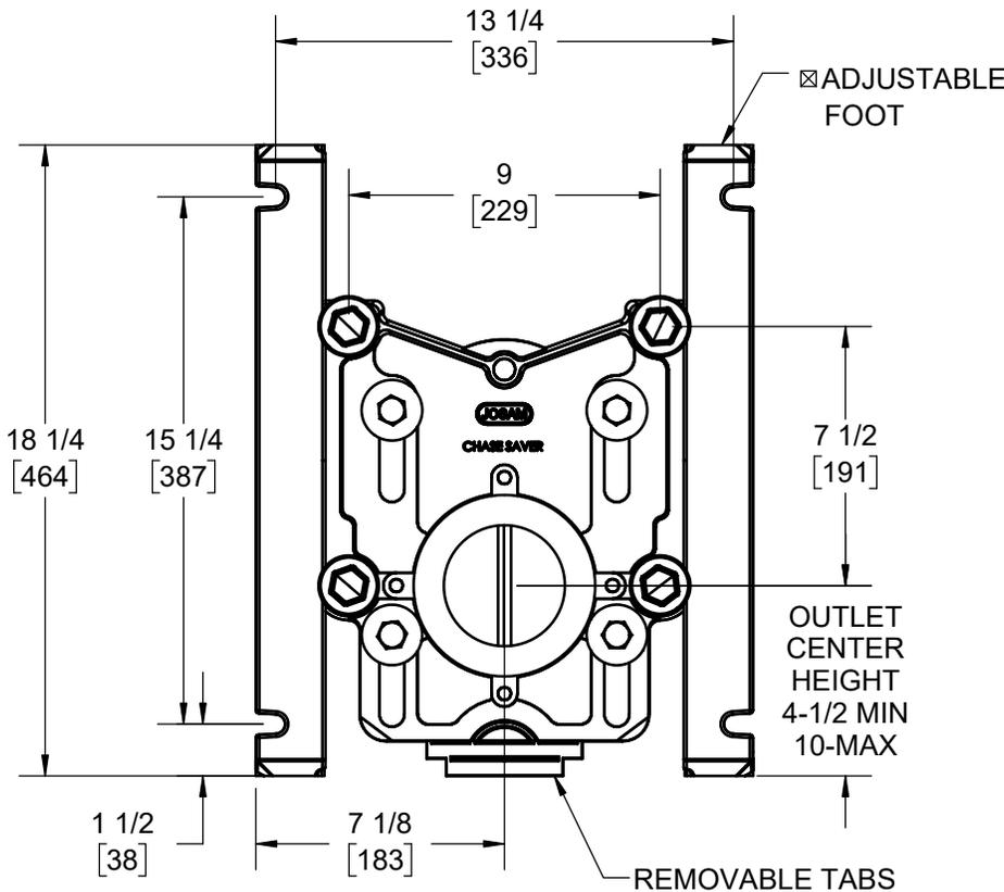
☒ RECOMMEND FEET BE SECURED TO FLOOR WITH 1/2" BOLTS AND ANCHORS (BY OTHERS).
