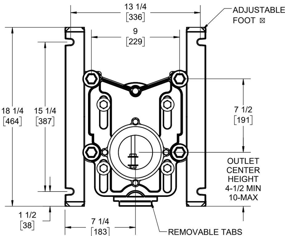
☒ RECOMMEND FEET BE SECURED TO FLOOR WITH 1/2" BOLTS AND ANCHORS (BY OTHERS).
